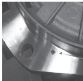
76% rejection (in Pareto) Due to Flange cut mark
